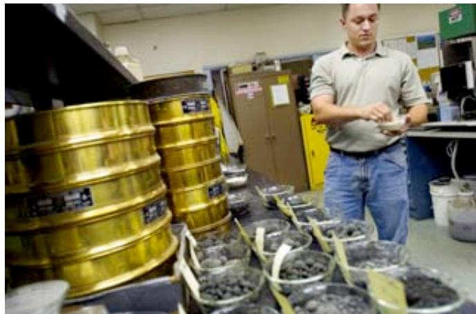
Morgan Johnson stands near where the clinker is tested for its chemical compounds in the lab at the Lehigh plant.
