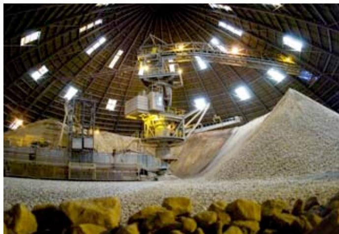
A radial arm, left, blends and stacks the raw material that will become Portland cement at the Lehigh Southwest Cement Co. plant in Redding. The limestone is crushed and cooked in a super-heated kiln, releasing carbon dioxide in a chemical reaction that forms the main ingredient in cement: clinker. Sacramento Bee/Andy Alfaro
