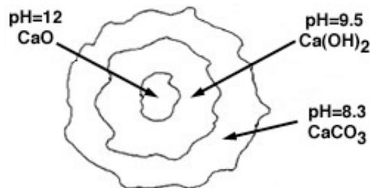
Diagram of a slag particle.
